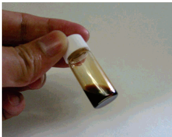
Figure 1. Photograph of a diluted surfactant solution (precursor solution) as an LLC former.
